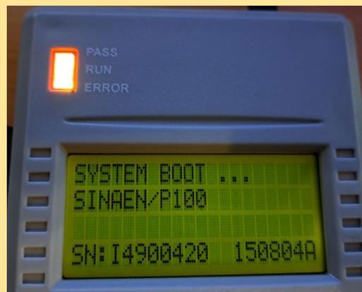
*When changing the authorization status (changing the second digit of the serial number) of the programmer, the first digit will automatically change to "0", which corresponds to SUPERPRO/IS01.*
