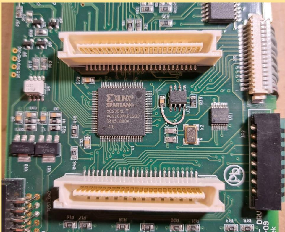
**Step5 – Solder two additional wires to the chip and keyboard connector**
